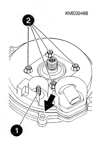
DISMANTLING AND CHECKING ALTERNATOR Dismantling cap Detach cap (1). NOTE: If stiff, prise off cap by applying suitable tool opposite regulator connection. Cap and bolts are always to be replaced.
